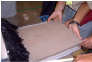
Fig. 4 A filter cake before microwave drying
