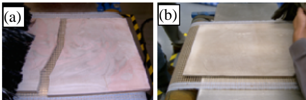
Fig. 5 A filter cake after microwave drying; (a) 15 mm. sample heated with 4 magnetrons (no. 2, 6, 10, 14) for 6 min, and (b) 8 mm sample heated with 2 magnetrons (no. 2 and 10) for 5 min.
